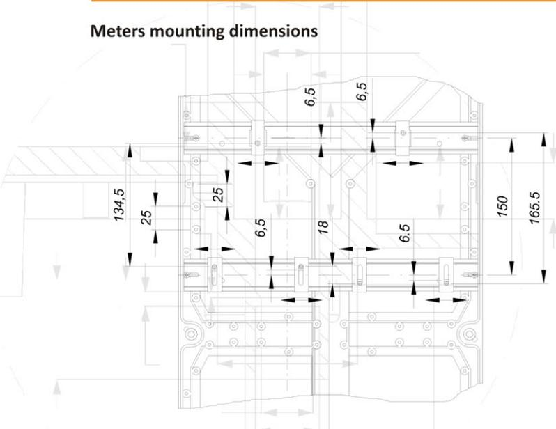
The meters are mounted on the enclosure base on rails W, by means of special M5 nuts, with degrees of freedom in two directions (or on flat rails with screws). This way of fixing allows various mounting dimensions for the meters. The drawing below shows the mounting dimensions for the meters, the distance between the Ω rails symmetry axes being of 150 mm.
